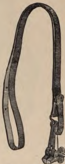
FIG. 234.—Portable vise with strap for pulling up the slack in splicing.
